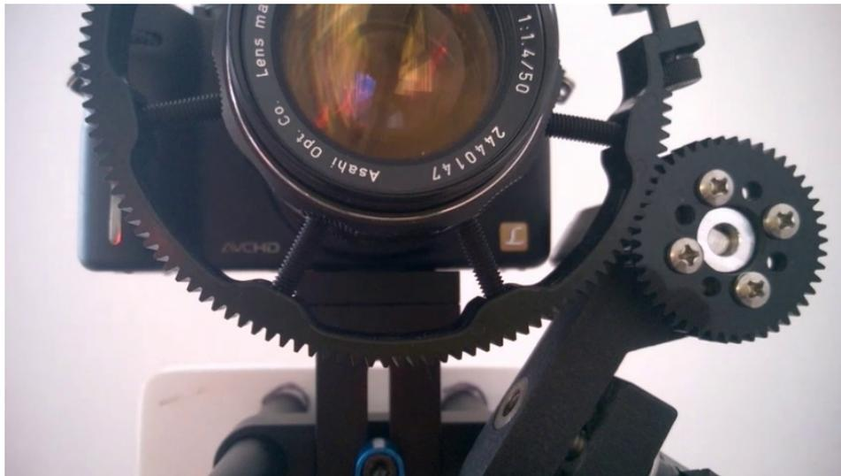
*Bracket Lensmotors, Lensgears and 15 mm rod system.*
